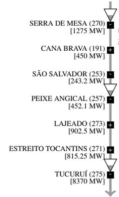
Figure 6: Basin map of Tocantins with power plant capacities. A plus, minus, or empty square corresponds to column SPAR-F in Table 3 and indicates a deterioration, improvement, or no change to the forecasts, respectively, relative to the PAR-F.
